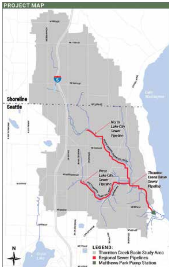
This map of the Thornton Creek Basin Sewer Study and Upgrade Project shows the study area along with the regional sewer pipelines.
