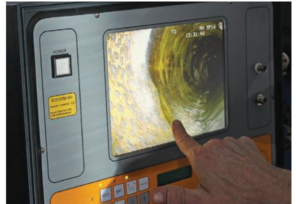
St. Helens Wastewater Utility worker Scott Williams points to a pipe defect on the Rausch monitor during a video inspection.
