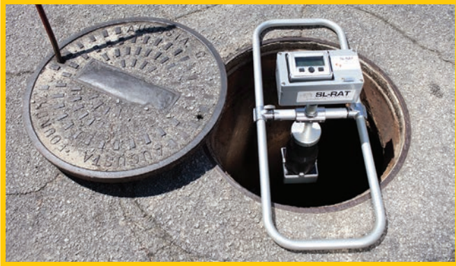
Traditional CCTV isn't the only means of sewer inspection. The Sewer Line Rapid Assessment Tool (SL-RAT) from InfoSense uses active acoustics to provide a quick view of pipe conditions.
