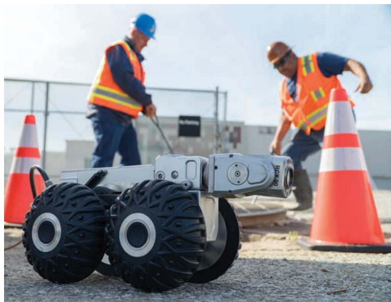
A crew prepares to launch an EnviroSight camera and crawler. Video inspection can pinpoint I&I sources after flow monitoring has established the most heavily impacted sections of your system.
