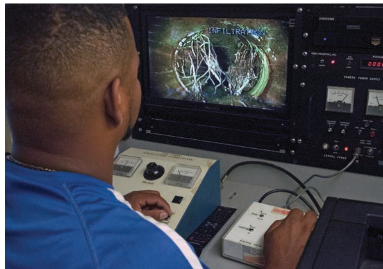
Darrell Noisette pauses to view an infiltration source while inspecting a sewer main on Sullivan's Island.
